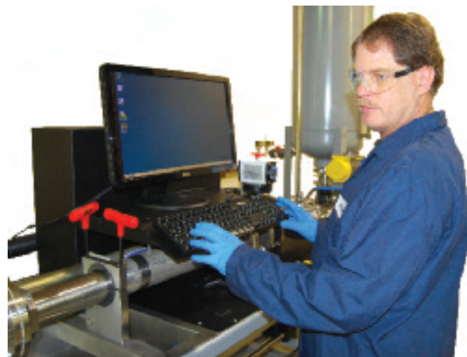
Operator is initiating Flo-Cal data acquisition system utilizing a user graphical interface. Flo-Cal controls the calibration process, both manually and automatically. It is also a diagnostic tool to present a graphic representation of the calibration, allowing for comparison of the previous calibration with the current calibration.
